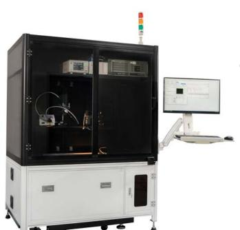
Optical path coupling inspection in silicon photonics wafer testing.
